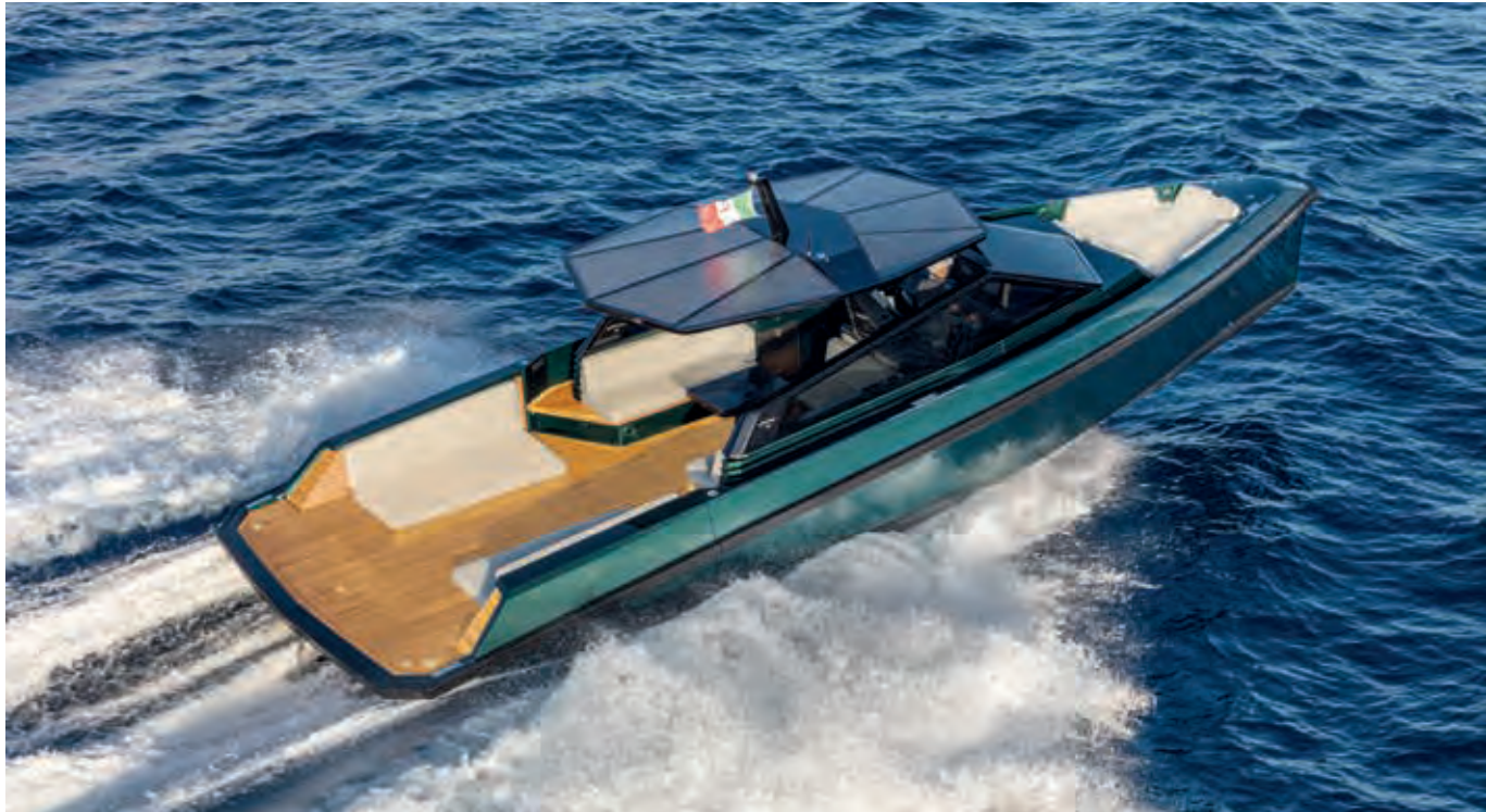
wallytender43 with solar panels on roof
