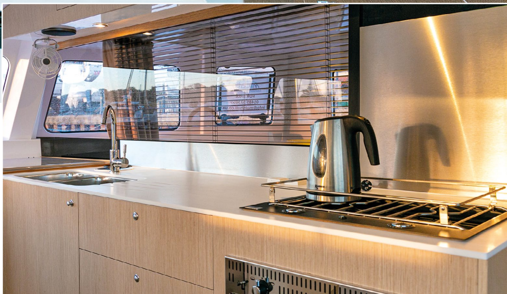
ABOVE: A simple linear galley to starboard adjoins the owner's cabin outboard. Gimbals are not needed for the hob or oven as they would be on a monohull
