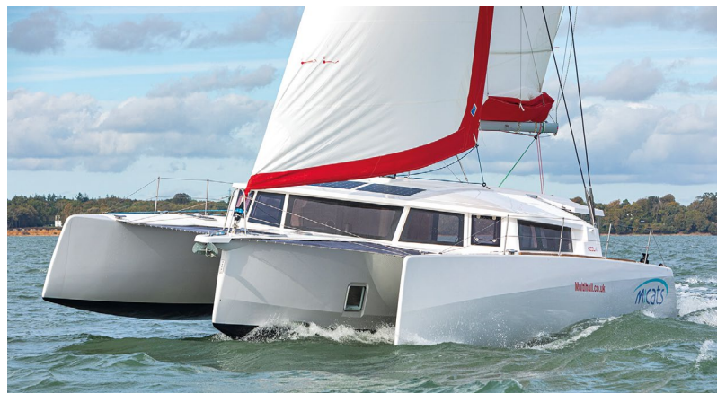
ABOVE: With one central keel and floats that clear the water, tacking is easier than on many catamarans
